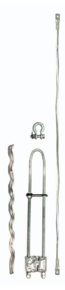
The Fiberlign Deadend is designed to terminate Optical Ground Wire (OPGW) while minimising any compression stresses that may be transferred to the core or optical elements within. The combination of retaining rods, wedge and housing distribute axial and compressive loading over a large area of the OPGW cable. Left-hand or right-hand lay style is provided to suit left-hand or right-hand lay OPGW respectively.
